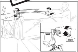
**Alternate tightening of the load carrier** Tighten a few turns, alternately on the left and right sides of the car. Press the tensioning tab against the car while tightening. Tighten firmly with hand pressure (corresponding to 4 Nm tightening torque).
