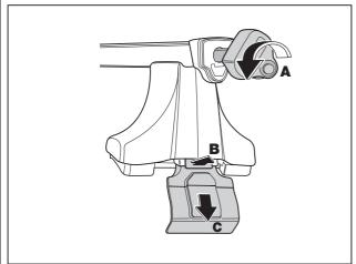
Removal/replacement of tensioning tab New car? Undo the tensioning tabs as in the illustrations.
