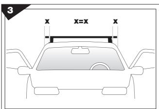
**Fitting the load carrier onto the vehicle** Wash and dry the roof. Open the doors. Carefully place the load carriers on the roof. The feet should be the same distance from the roof edge on both sides of the car (viewed from the front).
