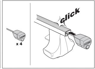
Slide the tightening knobs onto the bars until they snap shut. If you need to remove the knobs - refer to "To remove a tightening knob".
