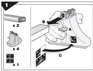
**First time assembly (A)** Raise the locking arms on the back of the load carrier feet and **(B)** slide the feet onto the bars. **(C)** To enable you to distinguish the front load bar form the rear load bar and the left-hand ends from the right-hand ends, use the decals provided to identify the feet.
